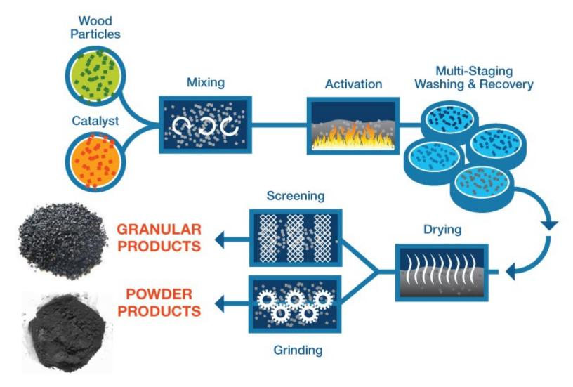
The wood particles are sawdust. The catalyst is phosphoric acid. No sewage sludge is used in the process.
